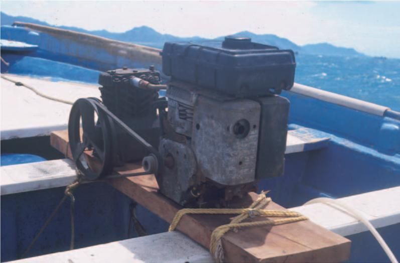
*Figure 3. Hookah air compressor used by Canal del Infiernillo divers.
